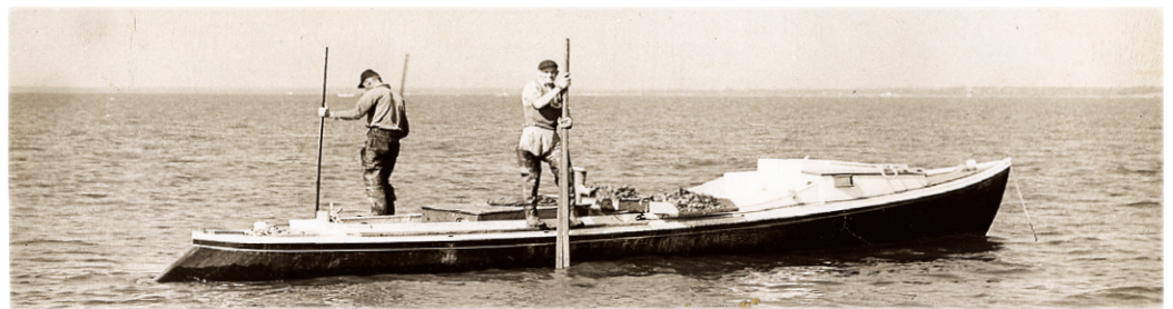
These oystermen are working off a deadrise boat with a Hooper’s Island Drake tail style stern. The photo was taken in the 1950s in the Rappahannock River.
