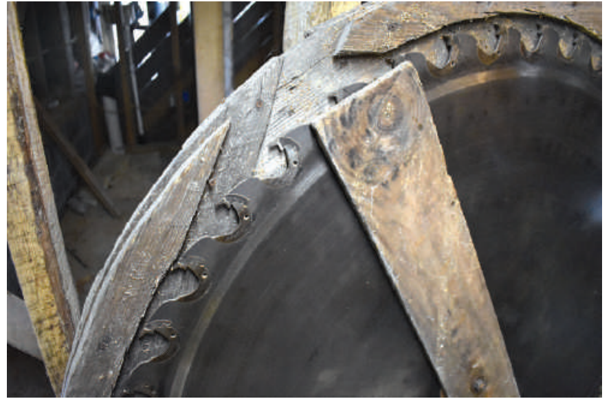
There are 54 teeth on the saw blade and all have to be, from time to time, professionally hammered for tension and shape.
