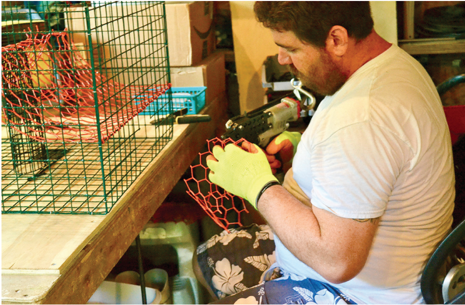
After Brandy Kennard bends the corners of the pot inward and cuts out the openings in the upstairs of the pot, he works on the funnels which he says are the hardest part of the process. Photo by AnnGardner Eubank
