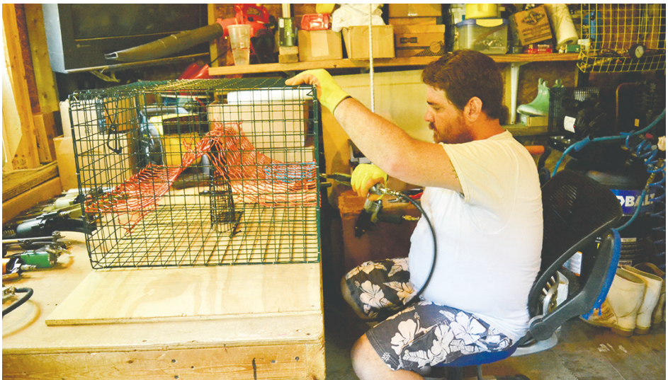
In his at-home work space, Brandy Kennard has a variety of tools he uses to make the process more efficient. Here, he uses a tool to bind the edges of the pot together. Photo by AnnGardner Eubank
